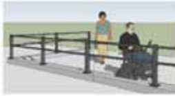
PEDESTRIAN CHANNELIZATION ON CURB OR KNEEWALL
